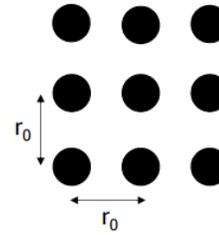
$$\text{Stress per bond/atom } (\sigma) = F/r_0^2$$
