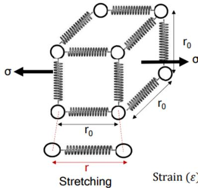
$$\text{Strain } (\epsilon) = \frac{r - r_0}{r_0}$$
