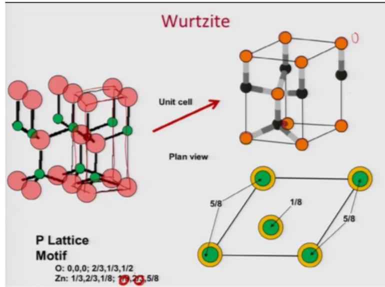
So moving on to the next one, this is where we see their structures. So, we have a hexagonal arrangement of cations. So, you can see that if I just change it to so here what you have is, so these are all; this is the first layer of anions. This is the second layer of anions and this is the third layer of anions. So, this is a b a; between these tetrahedral interstices are filled in such a manner, so that only 50 percent of them are filled.
