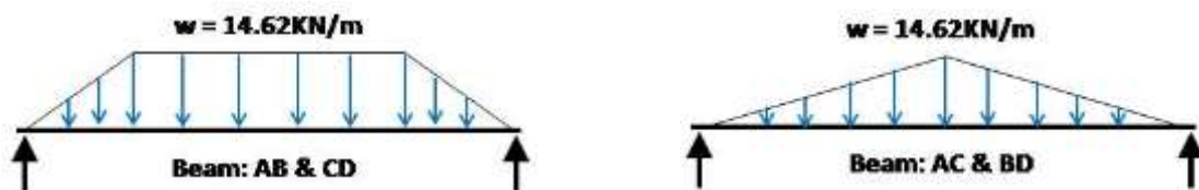
Figure 20 Load share in each of the beams
